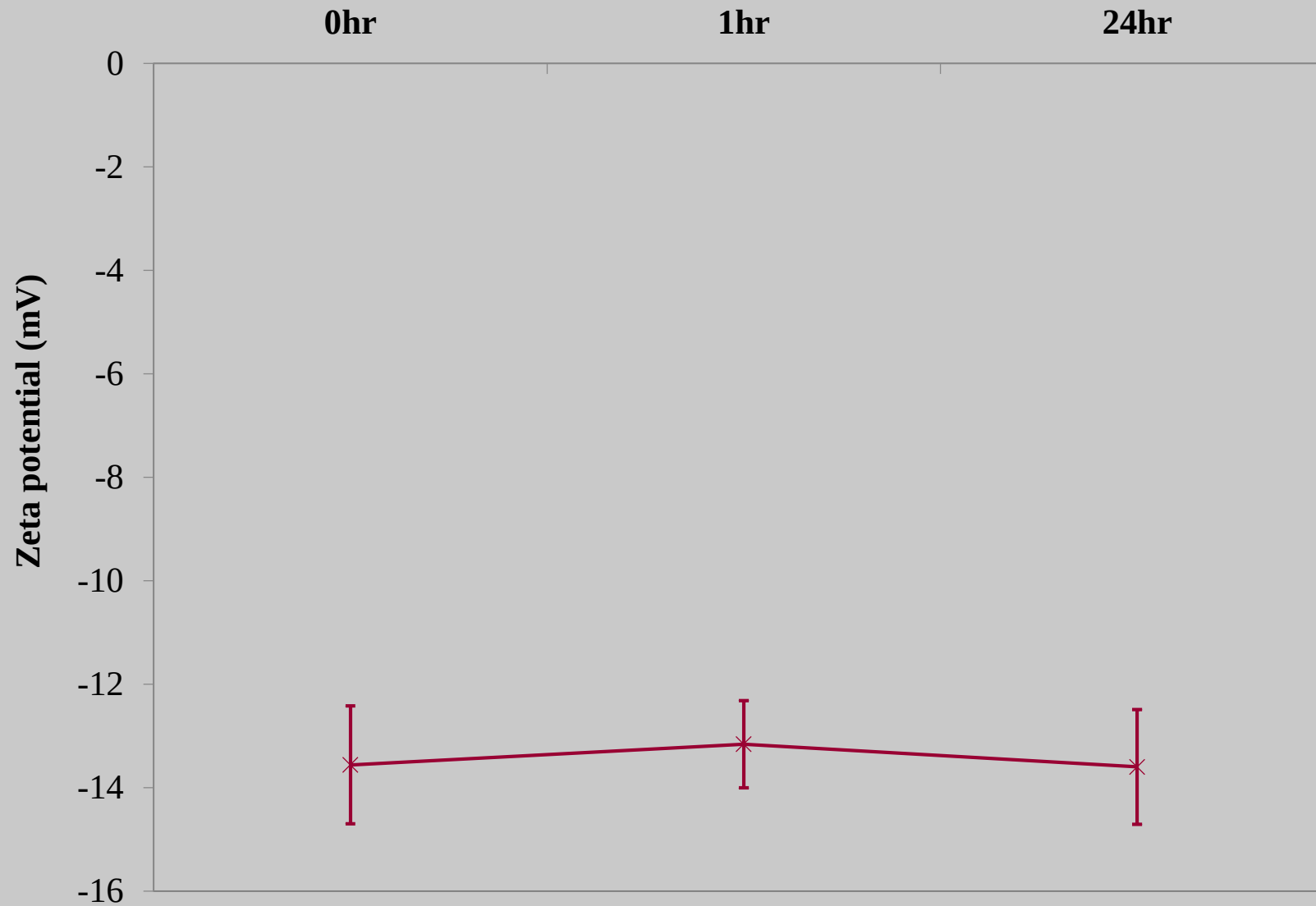
Fig 14: Zeta potential measurements of Adju-Phos in R10 medium following 0, 1 & 24hrs incubation (37°C). Error bars represent the \pm SD where n = 5 .
